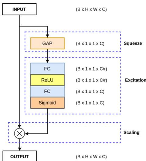
Fig. 4: Squeeze-and-Excitation (SE) Block
