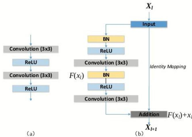
Fig. 2: ResUnet Basic Building Block
