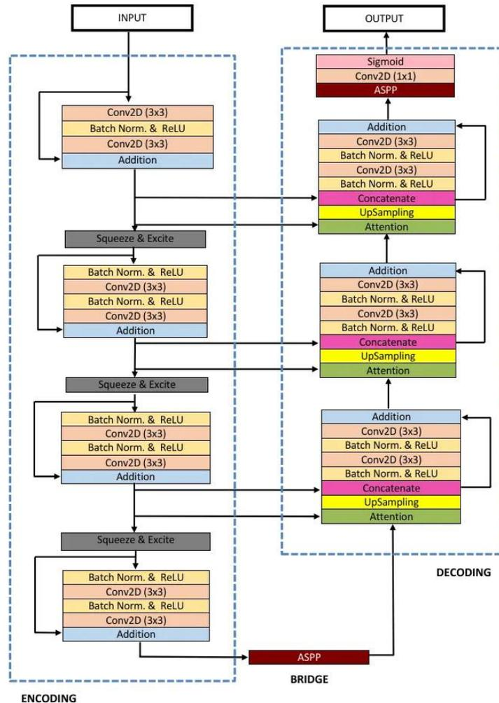
Fig. 3: Block diagram of the proposed ResUnet++ architecture
