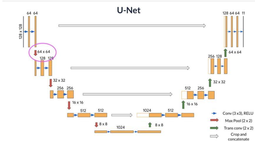
Fig. 1: UNet Models Architecture
